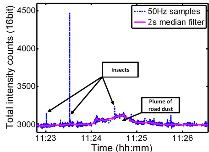
Fig. 3. The total scattered intensity over time, in the visible range, sampled at 50 Hz and with a 2 s broad median filter applied to the same signal, which is used to estimate the static signal. The positive fast spikes are caused by insects. Typically, the specimen passes the FOV in less than 50 ms. For comparison, the slow increase of scattering between 11:24 and 11:25 arose from a wide dust plume that was caused by a tractor driving upwind.
