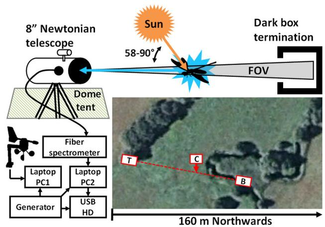
Fig. 2. Setup for the experiment. T: Newtonian telescope. C: Calibration site, B: Dark box termination. Light is collected by a 1mm UV fiber in the focal plane of the telescope and fed to a compact spectrometer. Distance from telescope to termination was 95 m of which the first 55 m cover grassland and the remaining 40 m cover the river Klingavälsån.
